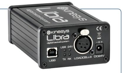
The **Libra Basic** power supply provides a simple and cost-effective method of powering the Libra Loadcell Shackles. When used in conjunction with the Libra Software loadcell data can be viewed, grouped and logged. A USB socket makes the connection to the PC very simple and the universal external power supply allows the system to be used anywhere in the world.
