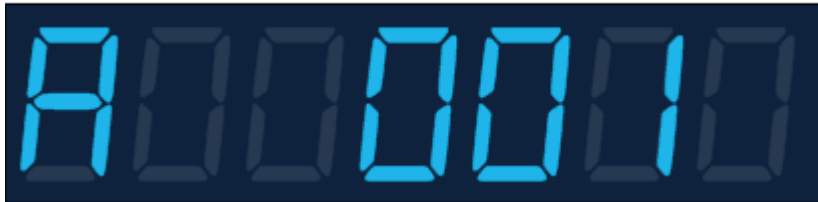
Elevation 1+ display showing address 1
