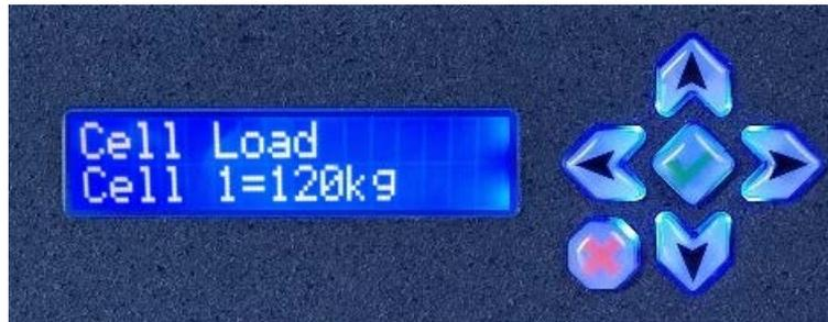
The LibraPRO display consists of four different display menus which are accessed in sequence by pressing the left or right buttons.
